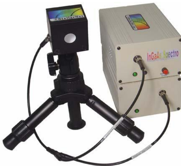
Figura 7. Spectrometrul StellarNet Dual Super Range 200-1700 nm
