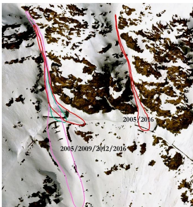
Figure 4.6.4: Avalanche events mapped for different years in the same area of Transfăgărășan highway on southern slope.
